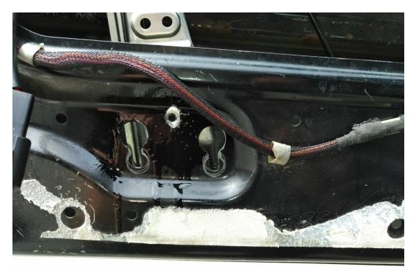
Once the hole is drilled, check the operation of the window making sure our regulator does not move side to side. If the hole isn't in the right spot, just find the correct spot and re-drill.
