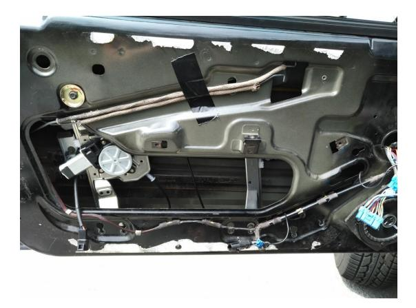
UPPER LEFT INSTALL - Use a large washer to make sure the left side of the regulator sits as high as possible in the stock mounting hole. This way the bottom of our regulator won't rub on the bottom of our door. Tighten slightly snug.
