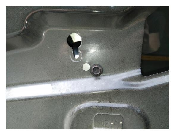
There's no guarantee that where my new mounting holes went will be the exact spot yours would go. Use the movement of the regulator as it's operated to find the correct placement.
