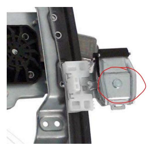
Fit the Cobalt regulator into the door frame with motor toward the trailing edge of the door. Two of the mounting holes in our door will work for two of the mounting points on the regulator. Using two of the bolts that previously held the old regulator in, attach the upper left and lower right of our new regulator. Using the adapter we made, attach the stock door harness of your jeep to the harness of the window regulator.
