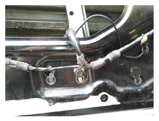
Reattach your window switch and check that your motor moves, Lower the window motor about half way so the bolts for the lifts are accessible through the door hole.
