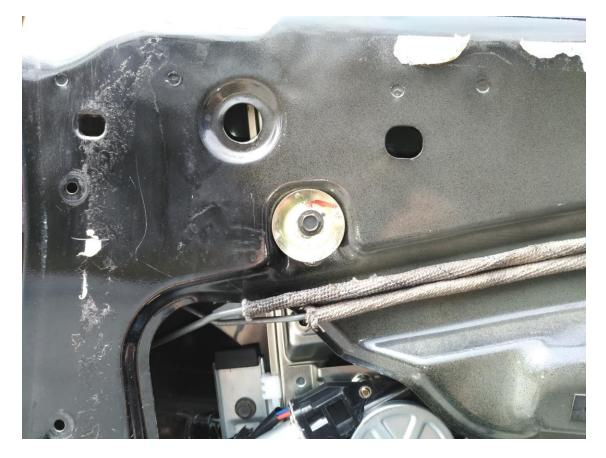
LOWER RIGHT INSTALL - Use another of our old 10mm bolts and washer to attach the lower right part of the regulator. It'll sit about in the middle of our right mounting hole. Use a washer to secure it in place. Tighten slightly snug.
