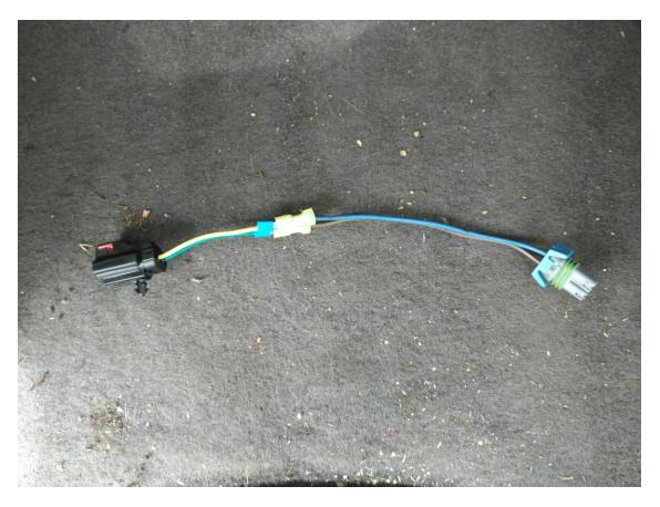
(NOTE: I used quick disconnect fittings in case the window didn't operate in the correct direction the first time. Do yours the correct way with butt connectors or soldering.)
